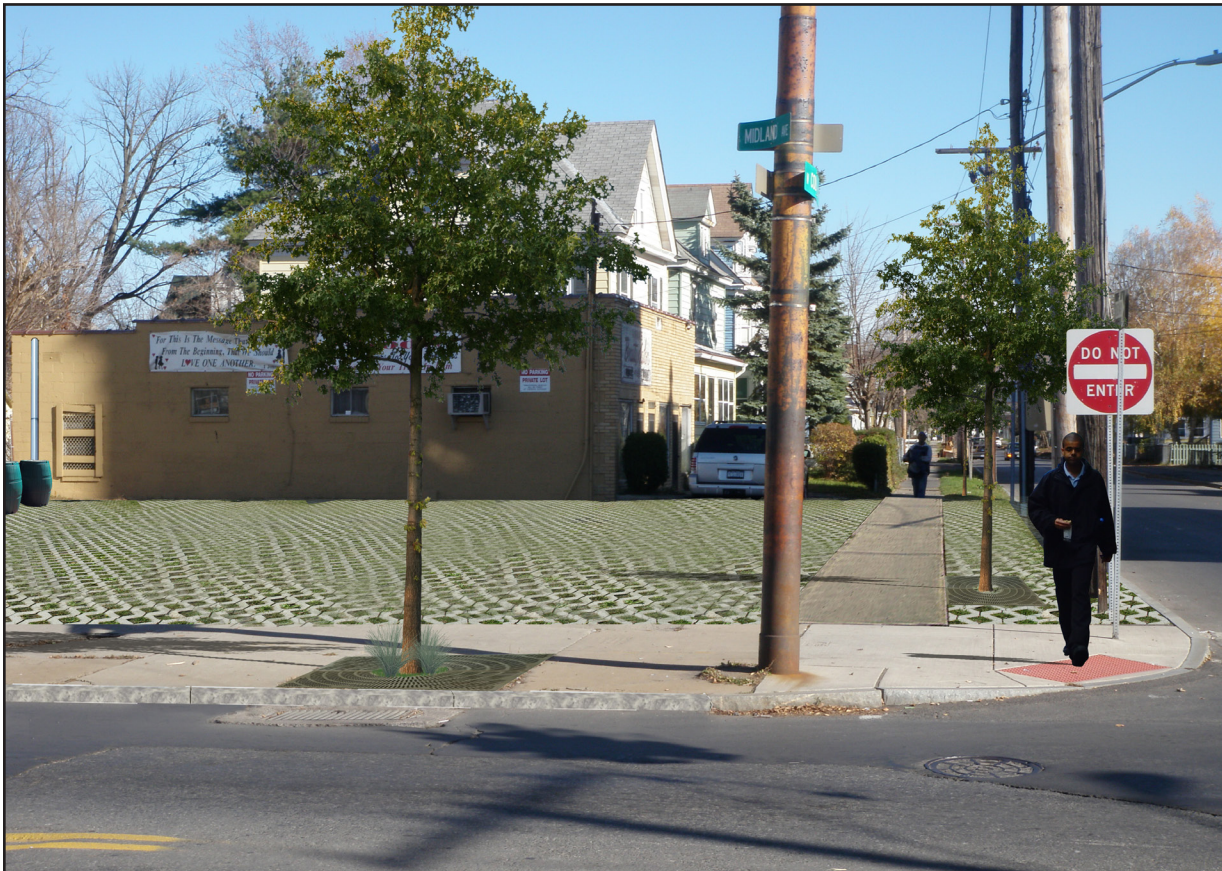
Photosimulation, showing pervious parking area, rain barrels, and tree plantings.
