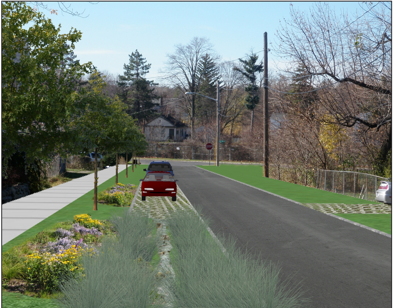
Photosimulation, Crehange St. showing vegetated swale, curb extensions, and parking with pervious surface.
