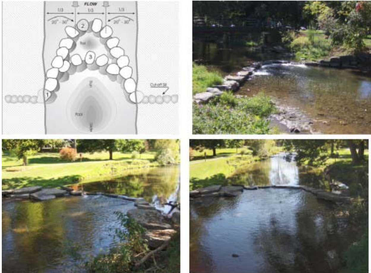
Figure 9: Cross-vanes in Nine Mile Creek at Marcellus Park. (Diagram Source: http://www.wildlandhydrology.com/assets/The_Cross_Vane_W-Weir_and_J-Hook_Structures_Paper_Updated_2006%20.pdf )
